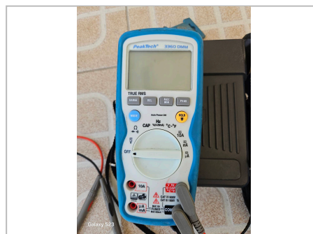
PeakTech 3360 true-RMS digital multimeter: second meter for cross-checking readings.
