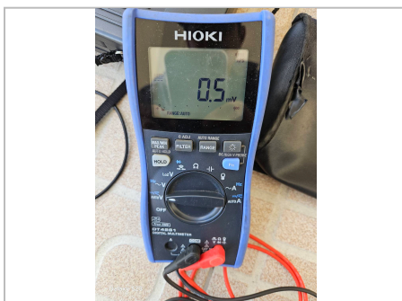
Hioki DT4261 true-RMS digital multimeter: AC and DC voltage and continuity checks.
