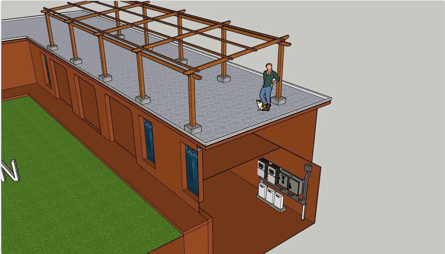
Frame only. Bare frame before the panels go on. Two lines of posts, with cross beams bolted on top and purlins running the full length.
